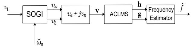
Figure 3: Adapted augmented complex least mean algorithm with fixed frequency (A-ACLMS-FF) for frequency estimation in single-phase grids.
