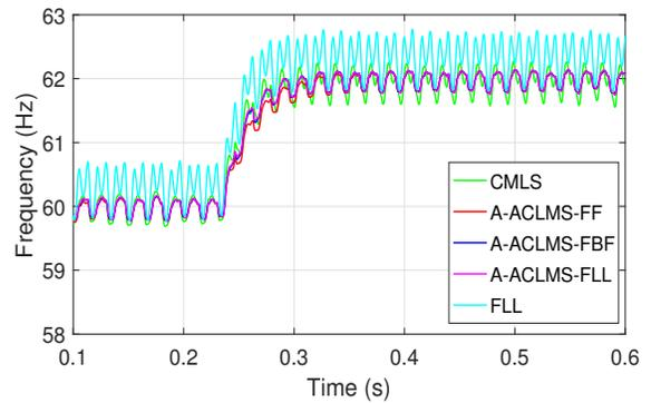
Figure 13: Frequency step in 0.23 seconds for a real signal.
