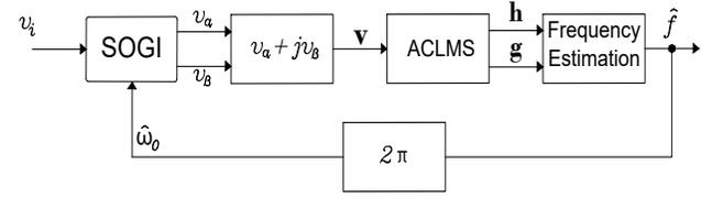
Figure 4: ACLMS feedback frequency (A-ACLMS-FBF) for frequency estimation in single-phase grids.
