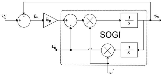
Figure 2: Second-order generalized integrator (SOGI) structure.
