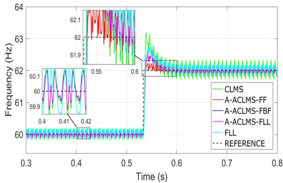
Figure 10: Frequency step in 0.53 seconds with harmonics.
