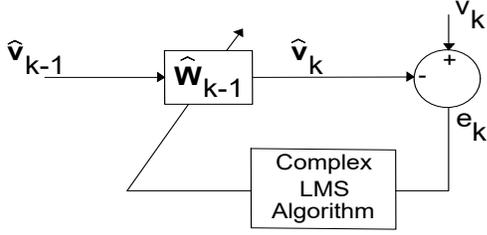
Figure 1: CLMS basic diagram.
