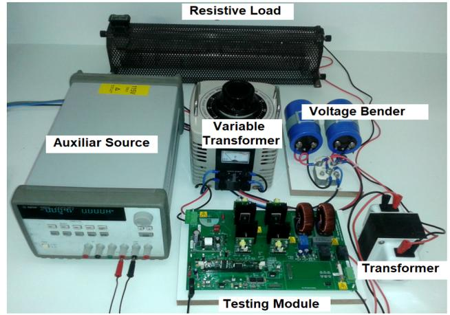
Figure 11: Experimental setup.
