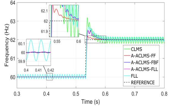
Figure 8: Frequency step in 0.53 seconds without harmonics.
