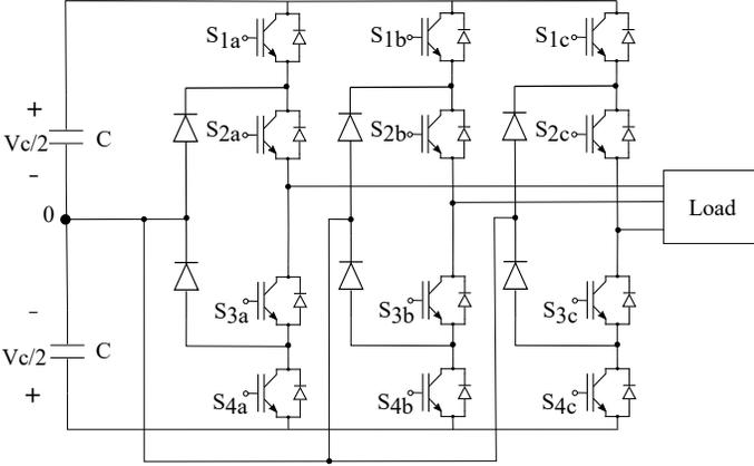
Fig. 2. Three-level Neutral-Point-clamped multilevel inverter.
