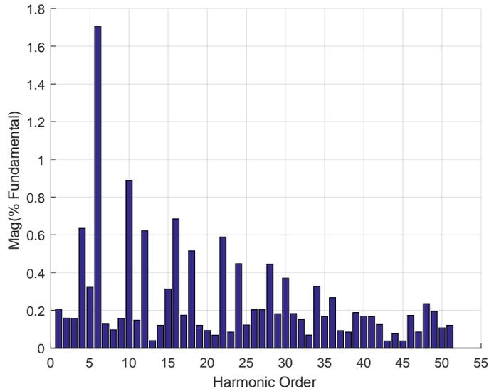
Fig. 11. Harmonic Distortion of  $I_g$  After Compensation.
