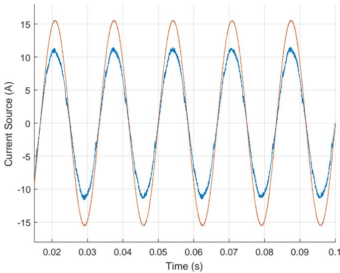
Fig. 8. Source Current After Filter Action.
