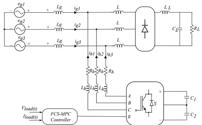
Fig. 1. Three Phase Parallel Active Filter.
