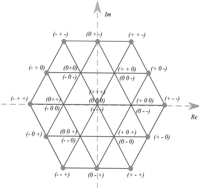
Fig. 5. Voltage vectors generated by NPC three-level converter.
