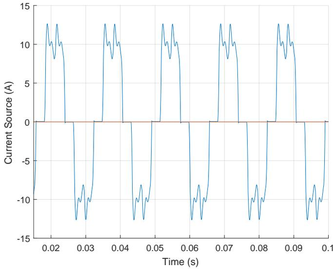
Fig. 7. Source Current Without Filter Action.
