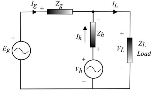
Fig. 3. Parallel Active Filter Mesh Model.
