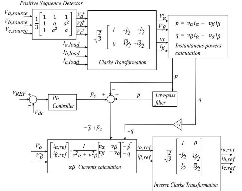
Fig. 4. Reference Generator Block.
